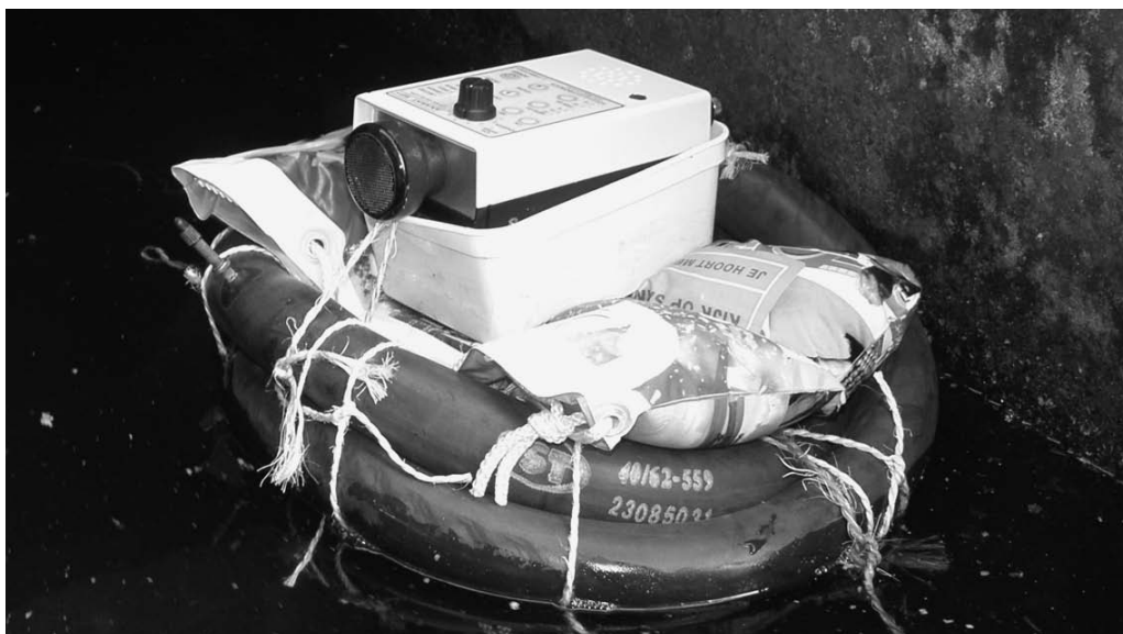
Photo 5. An Anabat detector, placed on a small raft. Photograph: M. Boonman
